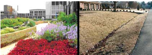
Figure 10. Water from a hardscape street diverted into a vegetation lined channel or "rain garden"
